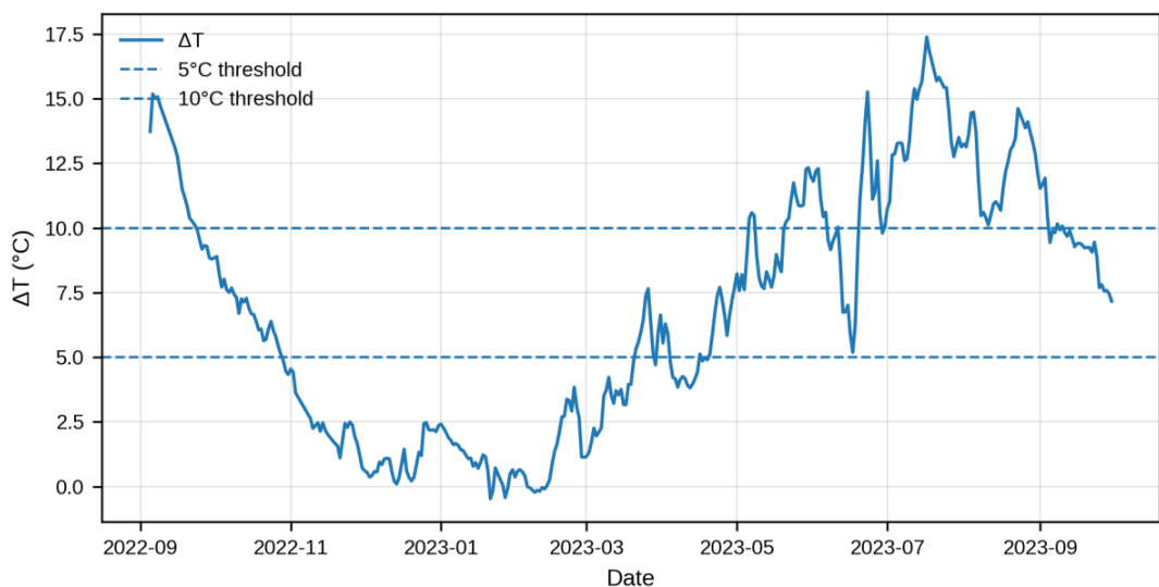
Figure 3. Daily stratification index \Delta T = T_{277} - T_{255} , with threshold lines indicating moderate stratification, \Delta T = 5^{\circ}\text{C} , and strong stratification, \Delta T = 10^{\circ}\text{C}
