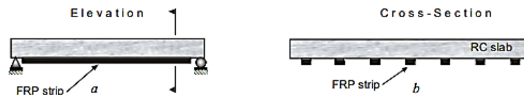
Figure 15. One-way slab strengthening, [22]
