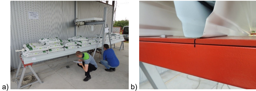
Figure 6. Specimen N8 B200: a) Arrangement of HPS under load p=2.5 \text{ kN/m}^2 b) support detail under p=2.5 \text{ kN/m}^2 , source: Authors
